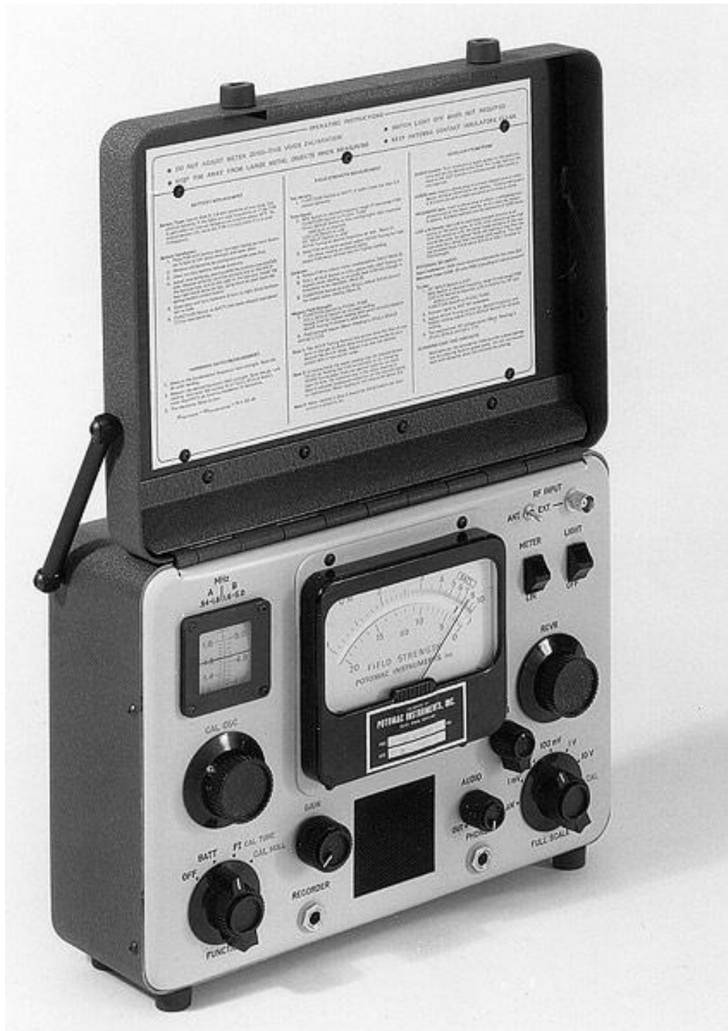
Figura 1. Field Strength Meter FIM-41
