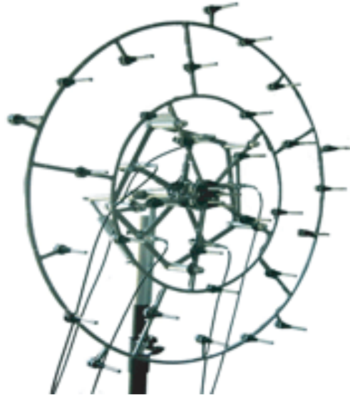
Figure 3. Plane Microphone Phased Array. Retrieved From: http://xn--42cga5ca0b6cdc2bzb3a7ble0ewa3nna3m.com/en/portfolio/microphone-array/ .
