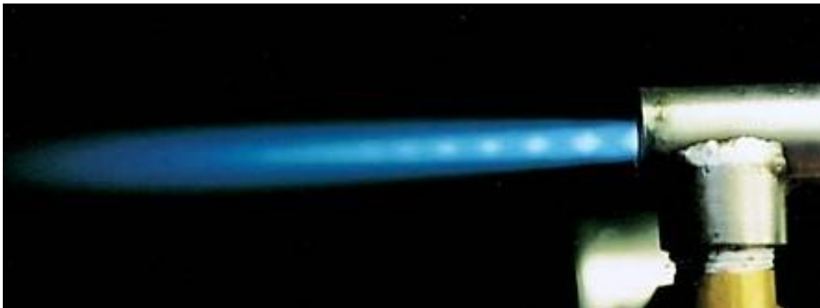
Figura 2.3 Diamantes Supersónicos HVOF (Linde Gas Division, 2009)
