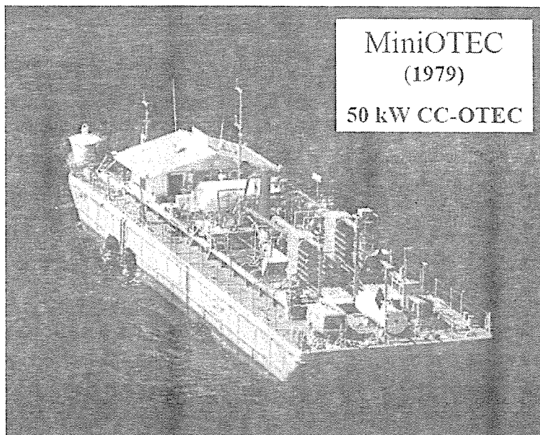
Figure 6: Floating CCS, 'Mini OTEC' off Keahole Point, Hawaii (Vega, 1999)
