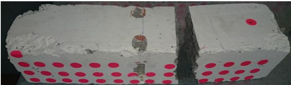
Fig. 19: Failure pattern for beam 8 at the side of the LDVT
