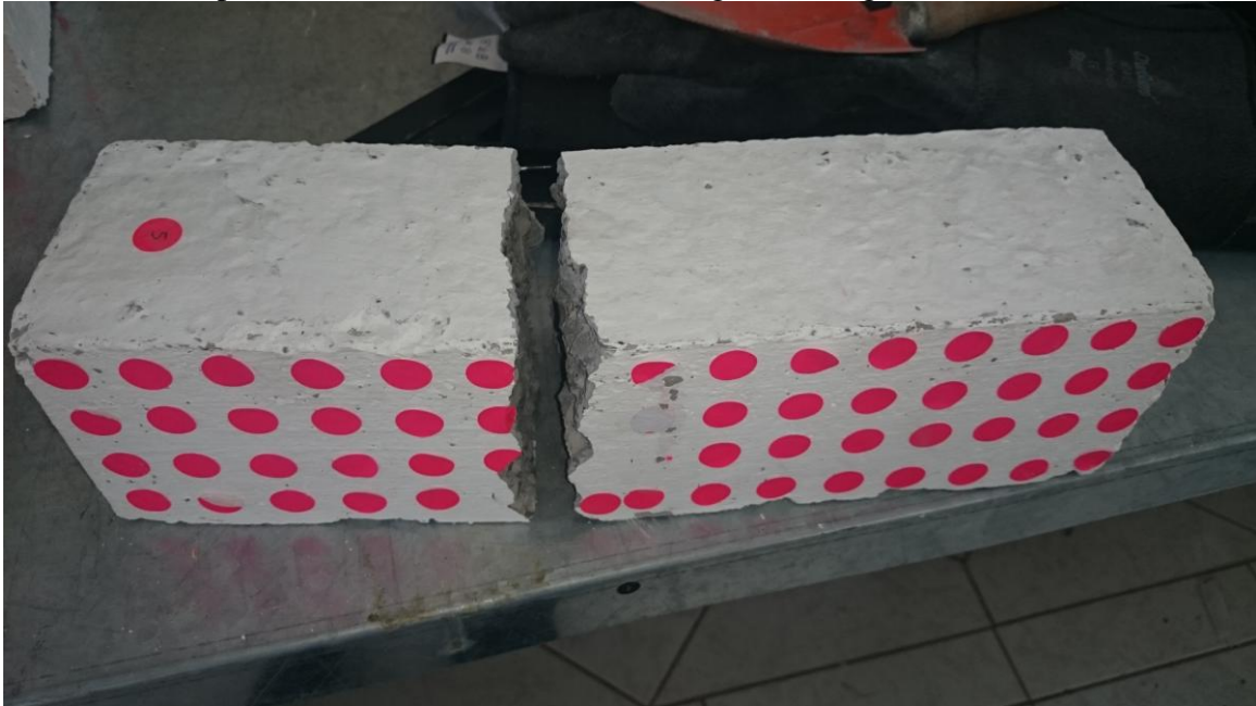
Fig. 13: Failure pattern for beam 5 at the side of the LDVT
