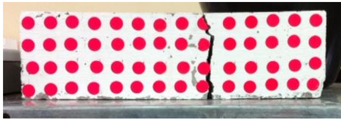
Fig. 10: Failure pattern for beam 4 at the side of the LVDTs.
