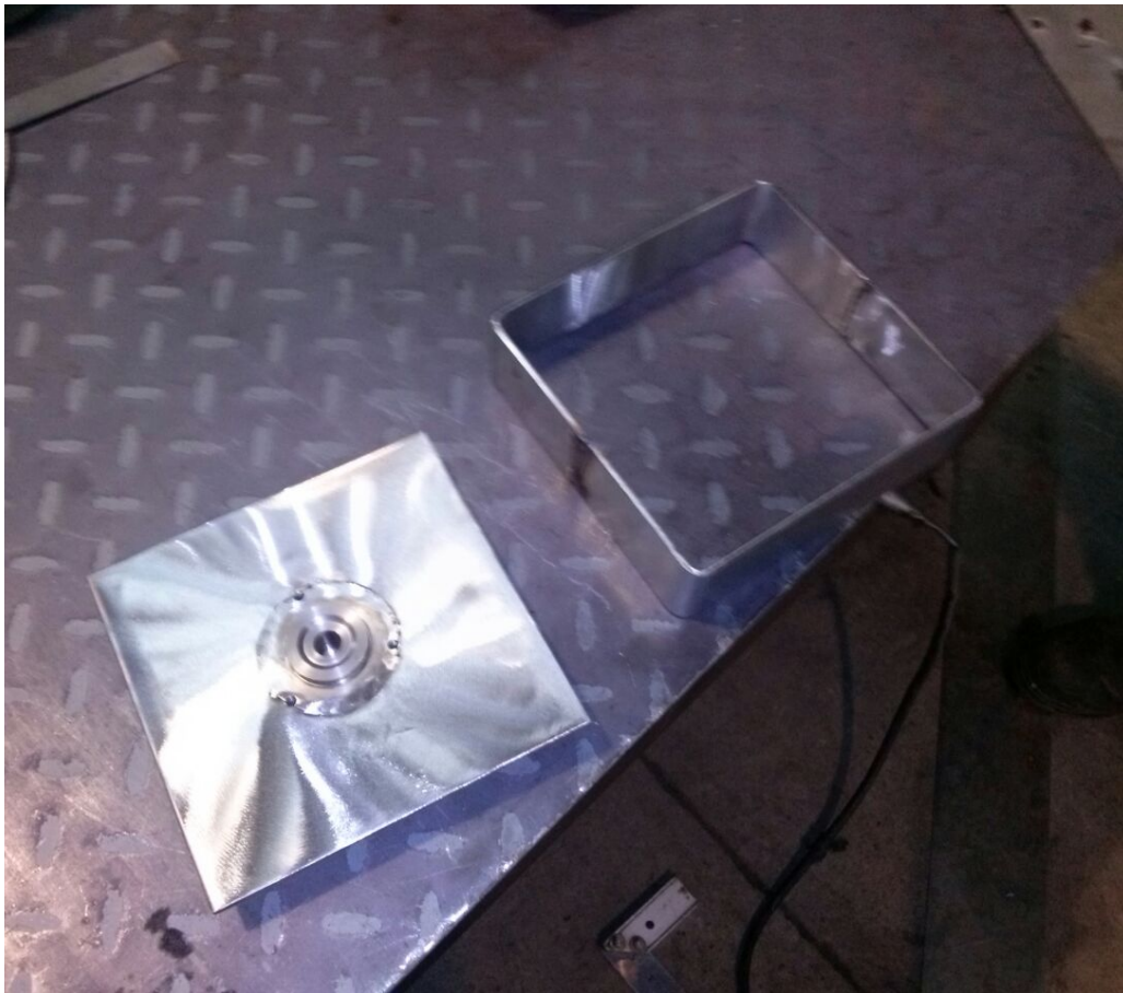
Figura 20: Pivote y base soldada
