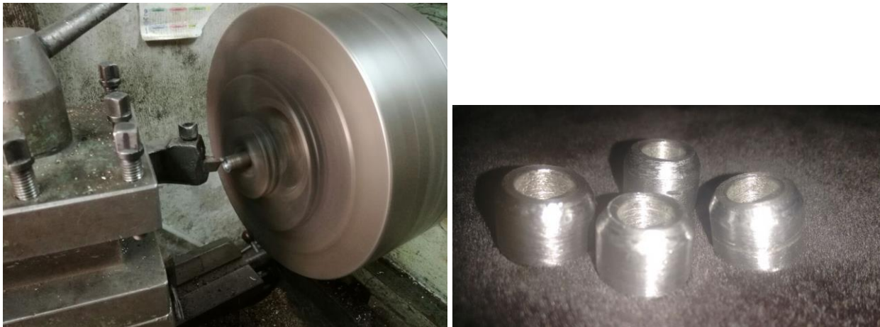
Figura 51. Manufactura de Pivotes
