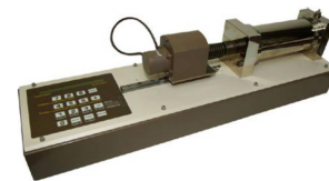
Fig 3. Advanced Pressure Controller used in Unsaturated Testing
