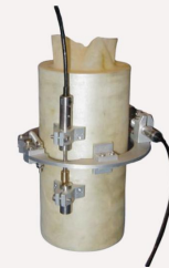
Fig 2. LVDT transducers as shown on sample.
