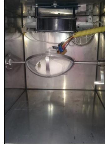
Fig. 14. Egg replica of an Andean Condor placed on the pivot with a 180 degree turn.
