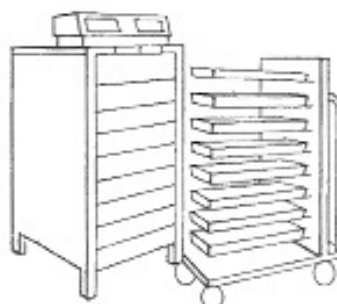
q Infrared (reethermic) oven system, 4.7 to 5.0 kW
