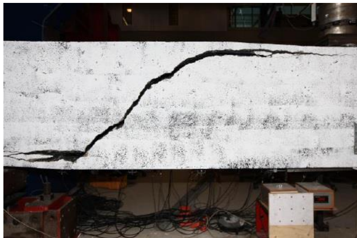
Figure 21 Failure of beam P804B after testing
