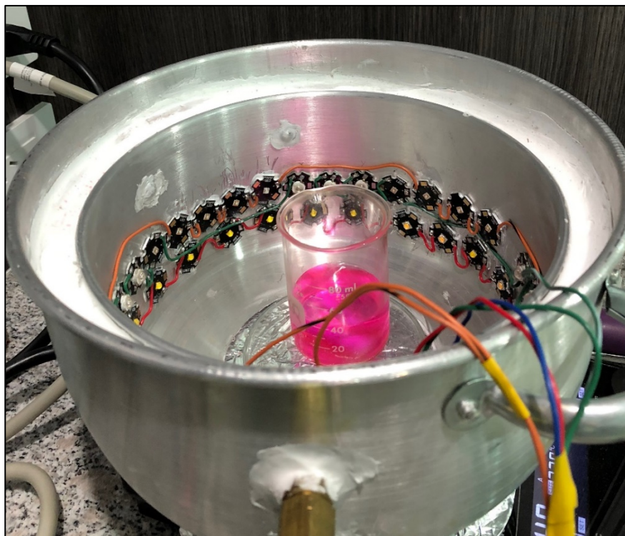
Figure 16: Constructed photo reactor for photocatalytic degradation of RhB, by Thomas Cadenbach
