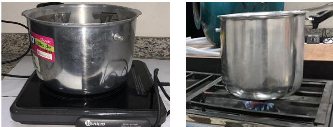
Figure 30. Energy efficiency test pressure cooker 2. Induction (left), Gas (Right).
