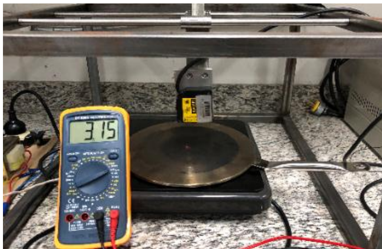
Figure 35. Deformation test. Stainless steel.
