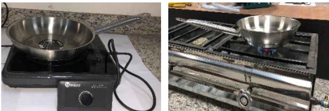
Figure 25. Energy efficiency test fry pan 2. Induction (left), Gas (Right).
