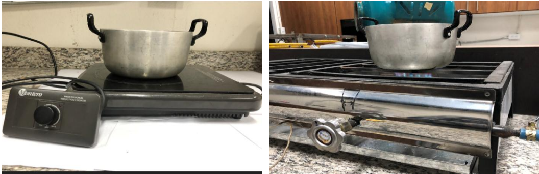
Figure 20. Energy efficiency test pot 1. Induction (left), Gas (Right).
