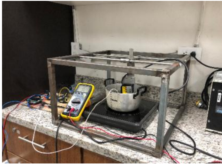
Figure 34. Deformation test. Aluminum coated with steel and stainless steel by metallization.
