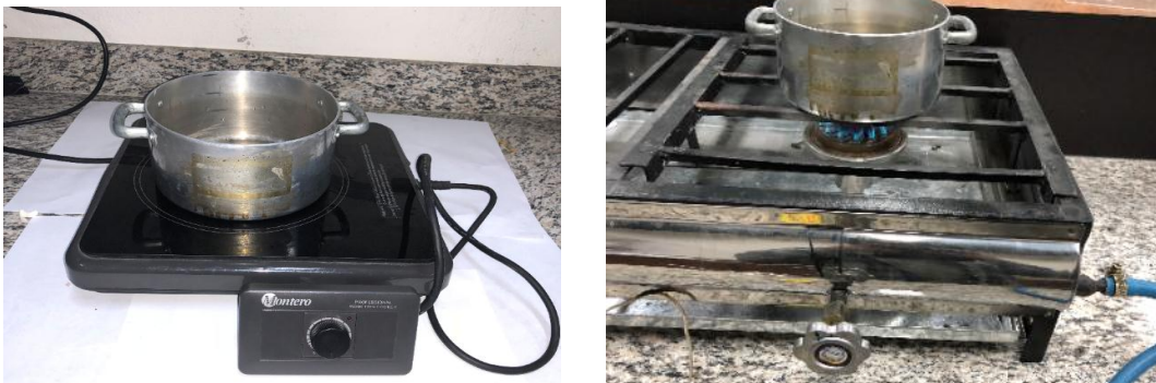
Figure 21. Energy efficiency test pot 2. Induction (left), Gas (Right).
