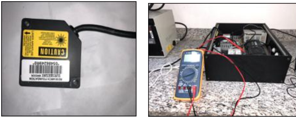
Figure 7. Position laser for deformation tests. Position Laser (Left), DAQ-3005 (Right).
