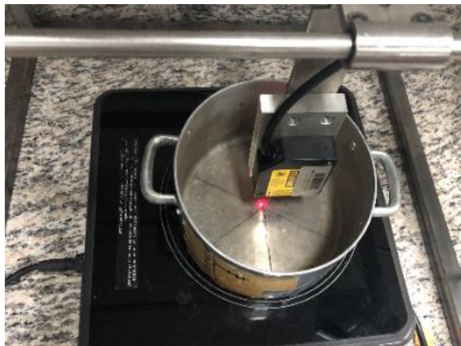
Figure 33. Deformation test. Aluminum with a stainless steel Incrustation pot.
