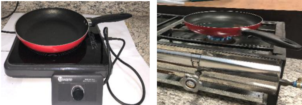
Figure 24. Energy efficiency test fry pan 1. Induction (left), Gas (Right).
