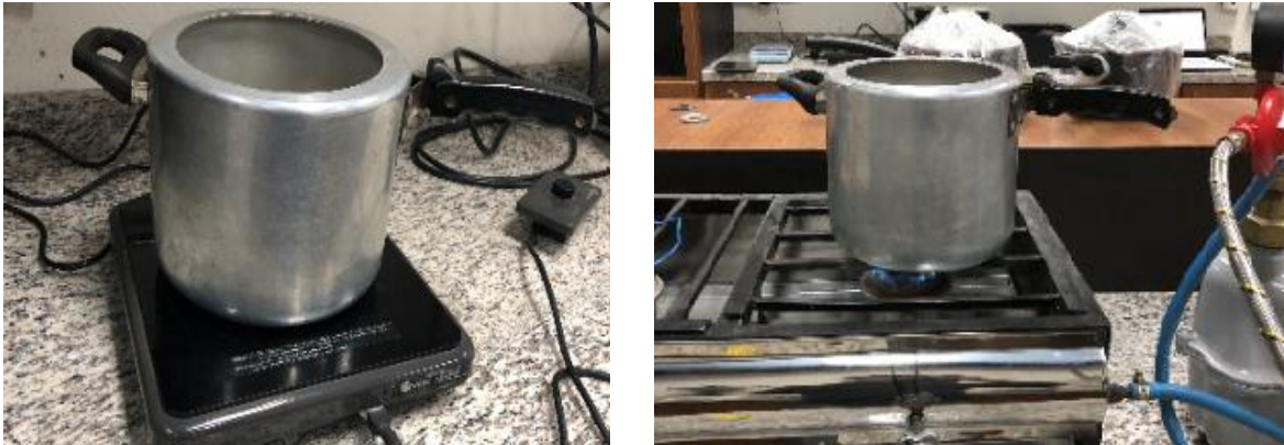
Figure 29. Energy efficiency test pressure cooker 1. Induction (left), Gas (Right).
