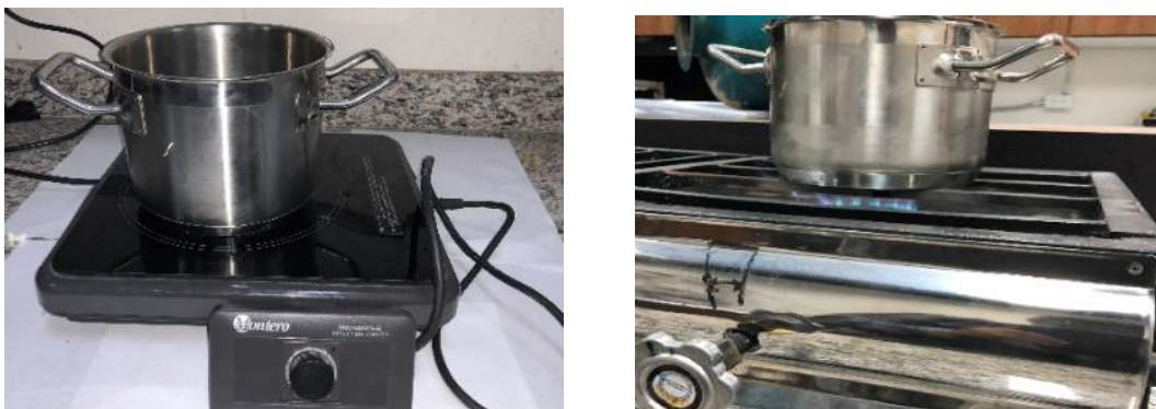
Figure 22. Energy efficiency test pot 3. Induction (left), Gas (Right).
