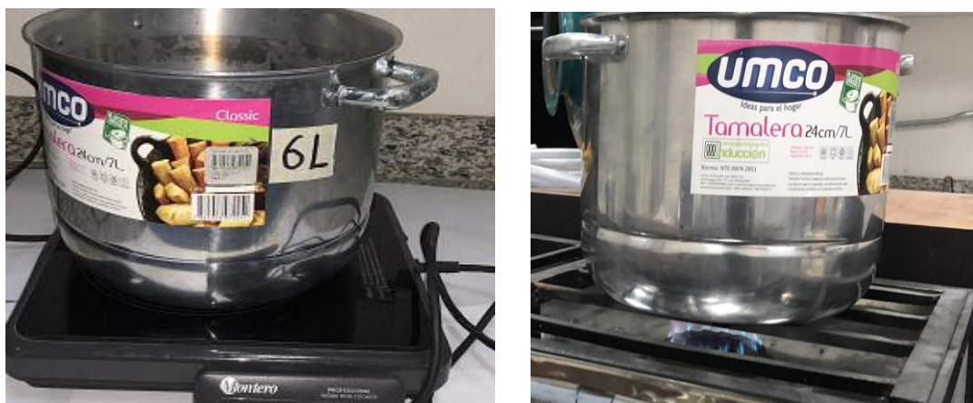
Figure 31. Energy efficiency test Tamalera 1. Induction (left), Gas (Right).
