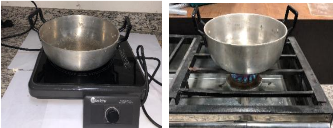
Figure 26. Energy efficiency test saucepan 1. Induction (left), Gas (Right).
