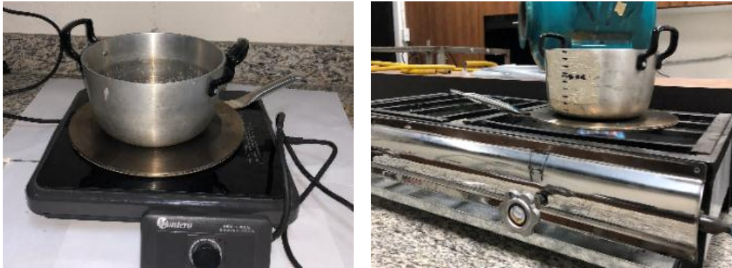
Figure 23. Energy efficiency test pot 4. Induction (left), Gas (Right).
