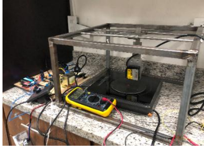
Figure 32. Deformation test. Aluminum with a stainless steel Incrustation plate.
