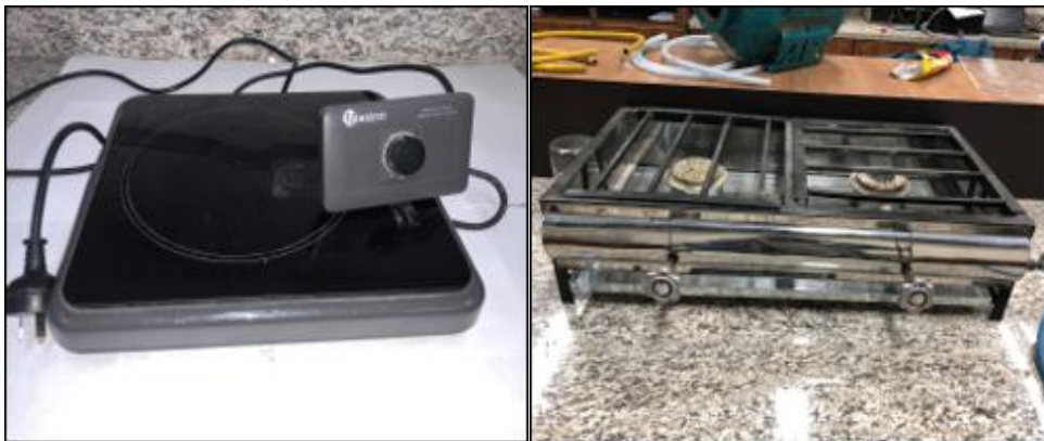
Figure 4. Stoves used for energy efficiency tests. Induction Cooker (Left), Gas Cooker (Right).
