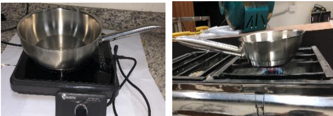
Figure 28. Energy efficiency test saucepan 3. Induction (left), Gas (Right).
