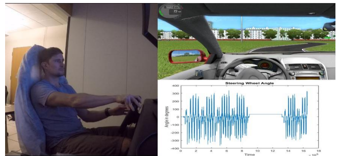
Figure 1. Experimental setup: (left) Participant driving in the simulator; (upper right) street view; (lower right) steering wheel rotation angular signal: right turn ( >0^\circ ), left turn ( <0^\circ ).
