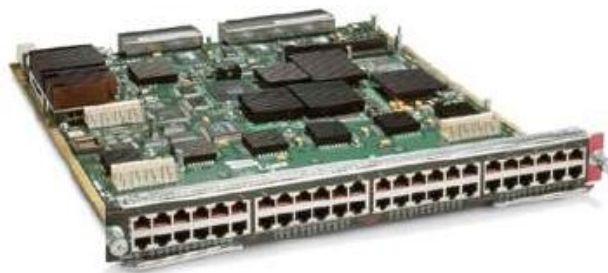
Figura 3.74: Tarjeta 10/100/1000 Ethernet de 48 Puertos
