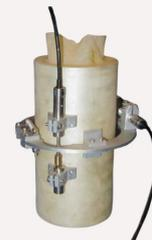
Fig 2. LVDT transducers as shown on sample.
