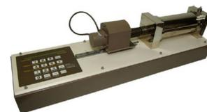
Fig 3. Advanced Pressure Controller used in Unsaturated Testing
