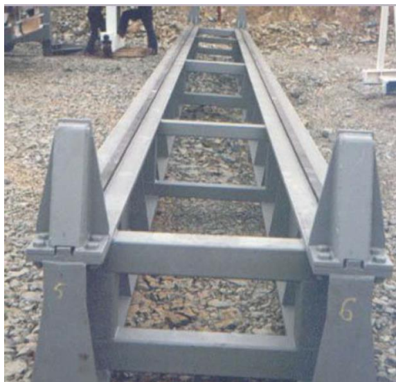
Figura No. 16: Vigas carril
