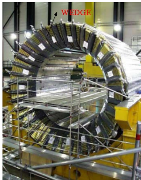
Figure 3. Isometric view of a complete half barrel of the HB HCAL (Barney, 2003)
