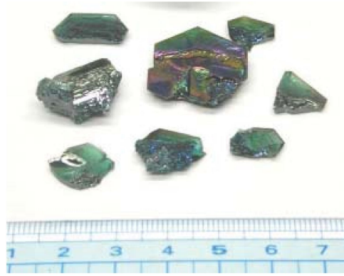
Figure 2.1: SiC platelets (mainly 6H-SiC) collected as a by-product in the Acheson process [5]
