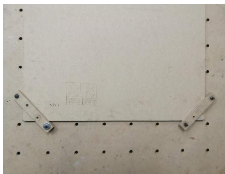
Figure 39. Workpiece secured into workspace.
