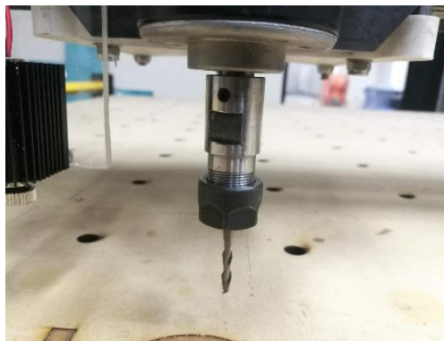
Figure 40. Milling bit close up.
