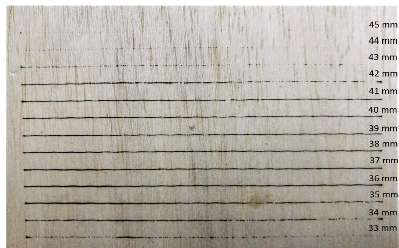
Figure 23. Engraving paths at different focal distance.
