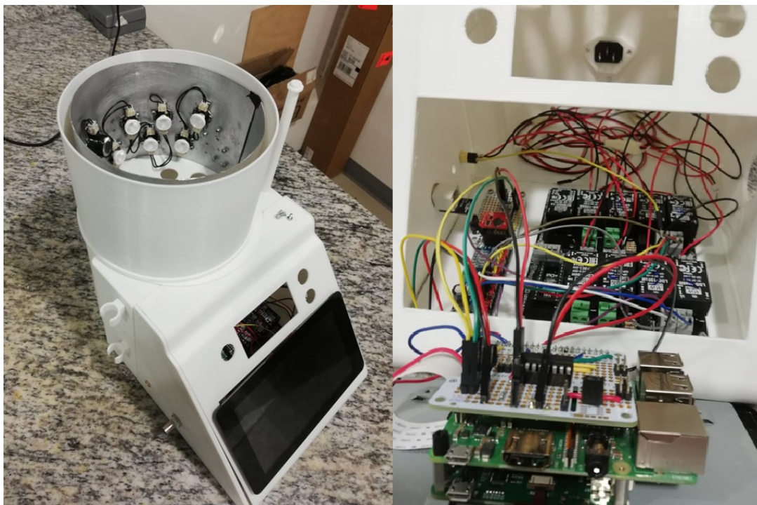
Figure 30. Construction of the Photo Reactor
