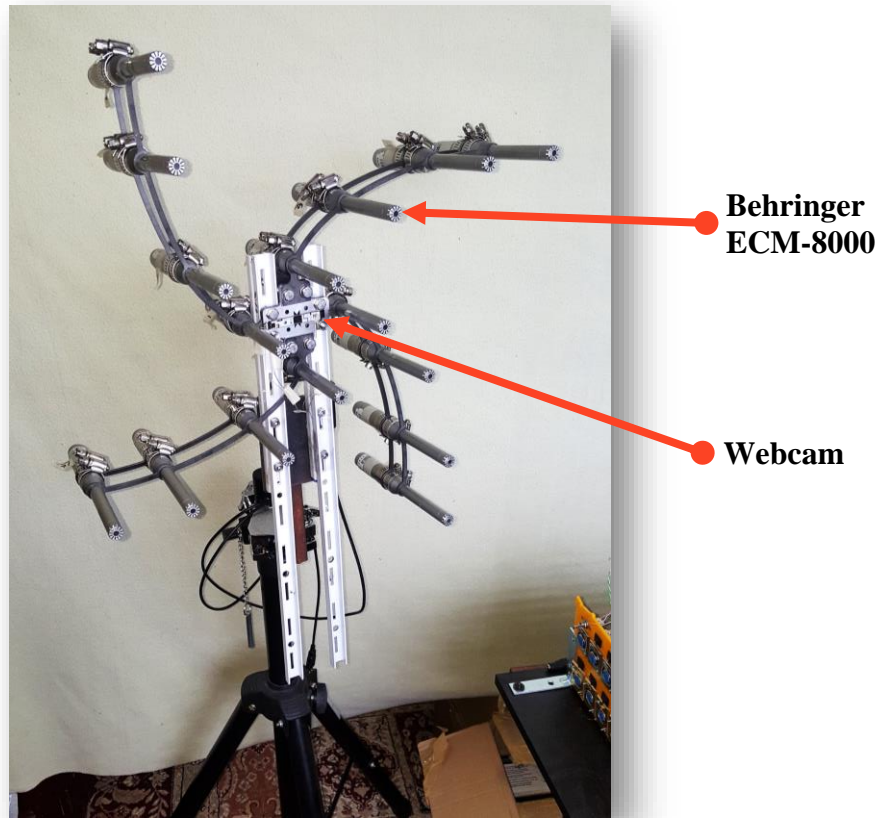
Figure # 6. Acoustic camera prototype built for this project.
