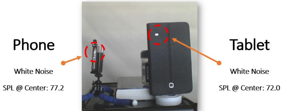
Figure # 11. Sound source set-up for test set # 2
