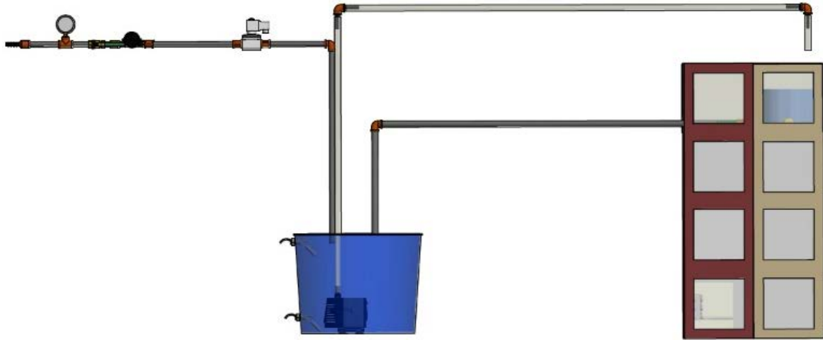
Figure 21: Water supply system.
